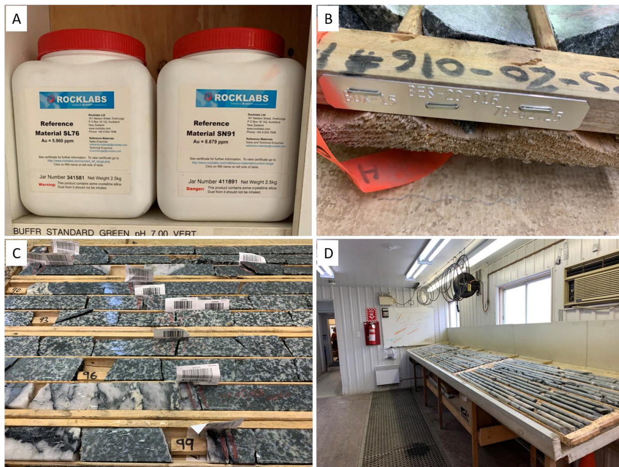
Figure 12-3: A) CRM storage; B) Core box with identification tags; C) and D) Core review in the core logging facility
