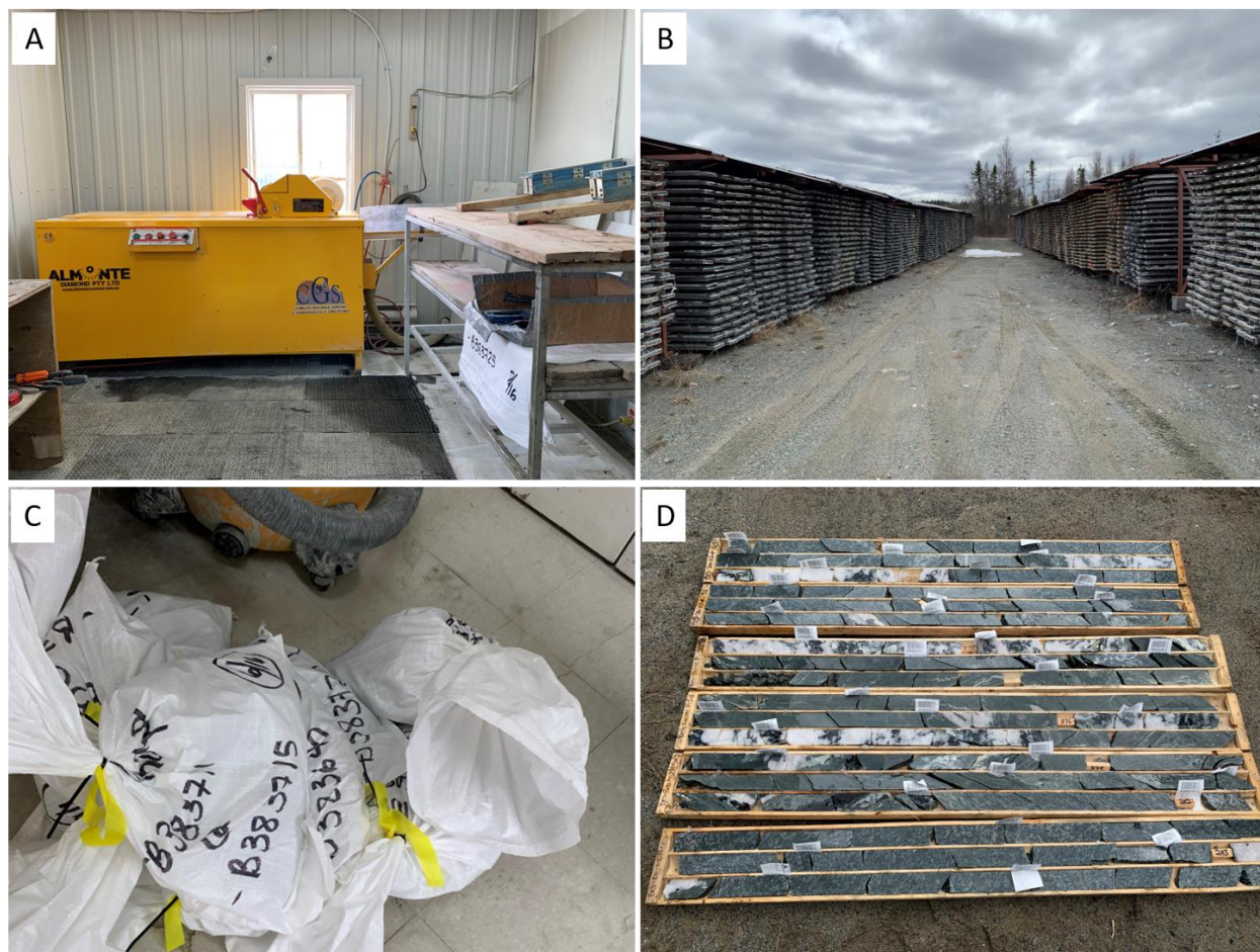
Figure 12-2: A) Sample preparation room; B) Core storage on site ; C) Samples ready for shipment to the laboratory; D) Mineralized zone half-core in storage
